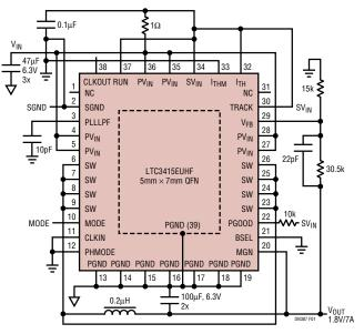
Figure 1. 3.3V to 1.8V/7A Application
