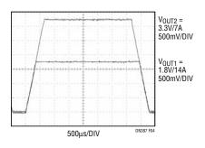
Figure 4. Output Tracking of Two LTC3415s
